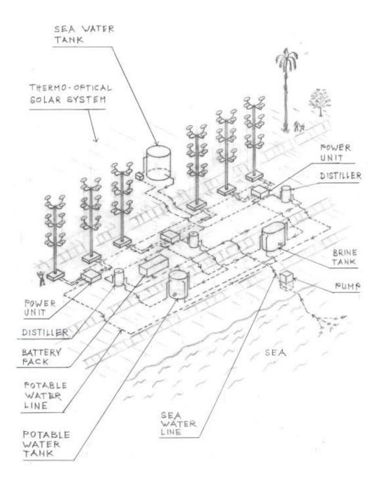
**FIG. 12** – Perspective View of a Modular Segment of the System for Harnessing Solar Energy, Potable Water, and Brine that can be used for the Extraction of lithium from the water of the Salton Sea, and other Coastal Cities.
