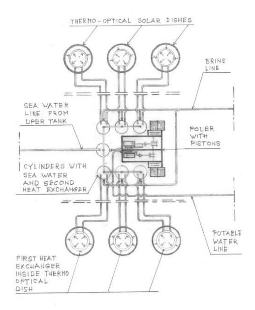
**FIG. 13** - Schematic Plain View of the Thermo - Optical Solar System (TOSS).
