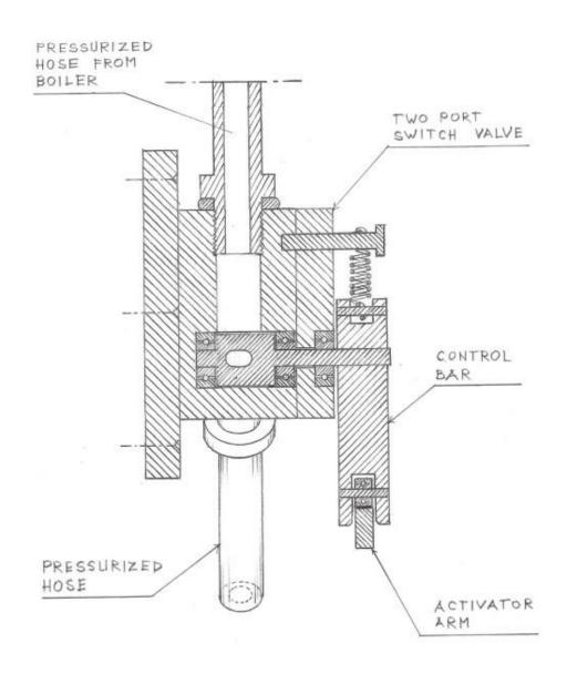
**FIG. 16** - Cross-Sectional View of Two -Port Switch Valve used in Power Unit with Pistons.
