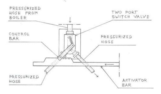
**FIG. 18** - Schematic Plain View of the function of the Two-Port Switch Valve - Stroke 2.
