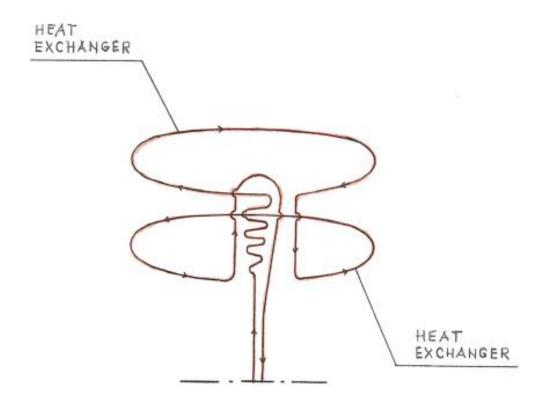
FIG. 6 - Schematic diagram of the flow of the synthetic oil through the heat exchanger of the Thermo-Optical Solar Dish
