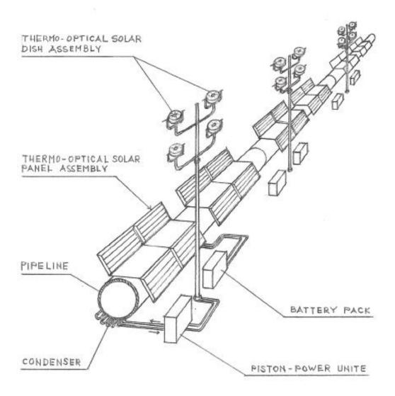
FIG. 1 - Perspective View of a Pipeline with Solar Panels attached to the Pipeline in combination with alternative Solar Dish System aside
