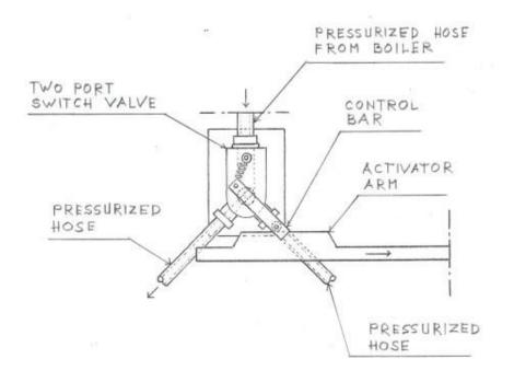
**FIG. 17** - Schematic Plain View of the function of the Two-Port Switch Valve - Stroke 1.
