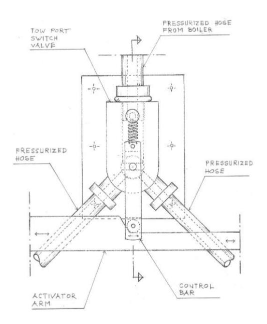
**FIG. 15** – Front View of Two -Port Switch Valve used in Power Unit with Pistons
