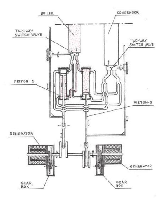
FIG. 9 - Schematic Diagram of a Piston Power Unit - stroke two
