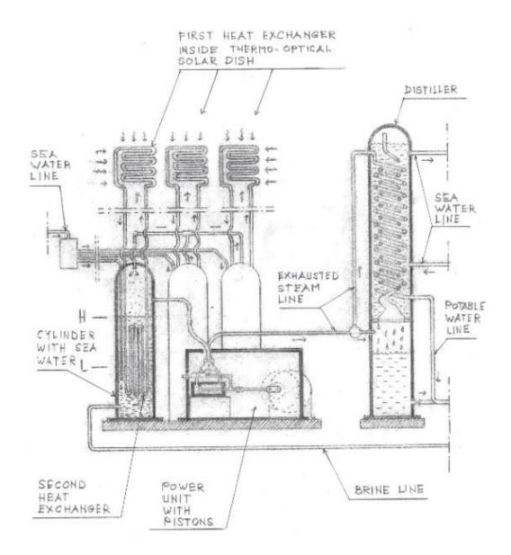
**FIG. 14** - Cross-Sectional View of the Thermo - Optical Solar System (TOSS).
