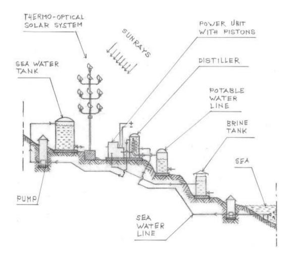
**FIG. 11** – Cross-Sectional View of a Modular Segment of the System for Harnessing Solar Energy for production Electricity Potable Water, and Brine that can be used for the Extraction of lithium from the water of the Salton Sea, and other Coastal Cities.
