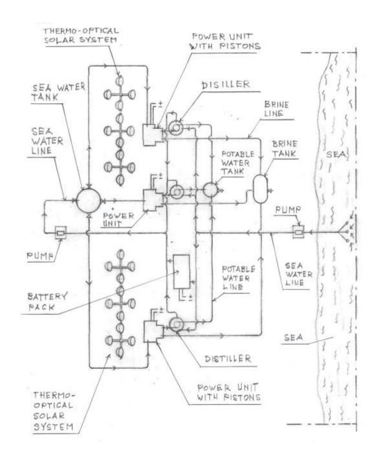
FIG. 10 – Plain View of a Modular Segment of the System for Harnessing Solar Energy for production Electricity, Potable Water, and Brine that can be used for the Extraction of Lithium from the water of the Salton Sea and other Coastal Cities
