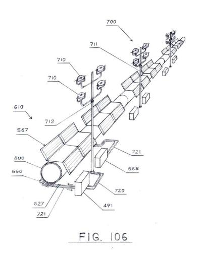
Perspective view of a pipeline with solar panel assemblies 610 attached to the pipeline in combination with a line of an alternative "thermo optical solar system" 700 aside pipeline.
