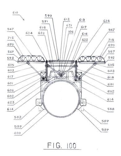
➤ A Thermo Optical Solar (TOS) panel assembly **610** and its attachment system to the pipeline **400**.
