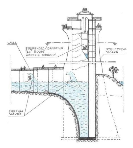
FIG. 11 - Cross-sectional view of a wave generation facility
